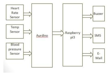
Fig.3 Patient health monitoring system - Block diagram
