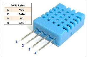
Fig.6 Temperature sensor
